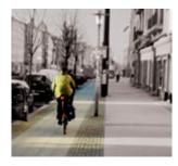
A cycle path is separated from the road by a kerb and from the pavement by markings, paving or a low kerb.
